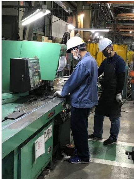
Panel repair process: Cutting out and bending
