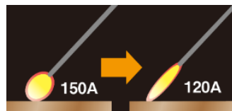
DROOP(Drooping characteristic) When the arc length becomes long and thus the voltage rises, the current decreases.
