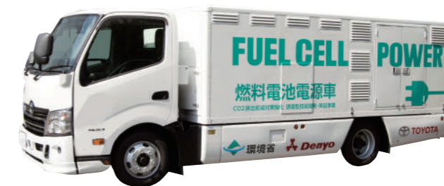
Power supply vehicle that uses hydrogen as a fuel to achieve zero CO 2 emissions during operation
